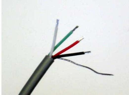
6. Crimp a terminal onto each of the wires (but not onto the shield or drain wire). Crimp each terminal using small needle-nosed pliers. After the terminals are crimped, solder the connections, taking care not to let solder run into the body of the terminals.
